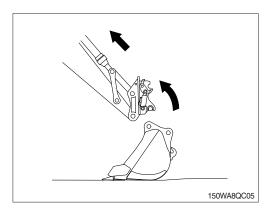
(8) Move the arm (1) and raise it until hook engages the upper (2) pin or interface of attachment.
