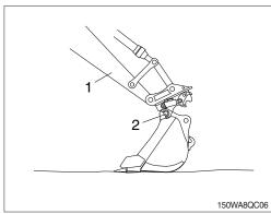
(9) With the bucket crowded, engage the quick coupler to the lower attachment pin or interface.
