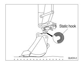
(4) Operate RCV lever to bucket-in position. Then, the moving hook is coupled with the bucket link pin while pressing the quick coupler switch. Make sure that the moving hook is completely contacted with bucket link pin.
