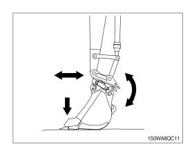
(14) Visually check that quick coupler is fully engaged and locked before operating the machine and attachment.
