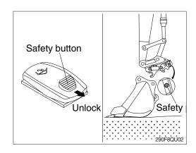
(3) Aligning the arm and bucket, insert static hook of quick coupler to the bucket pin while pressing the quick coupler switch.
