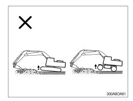
Excessive force as above may also result in vibrations being transmitted to the tracks causing damage.
